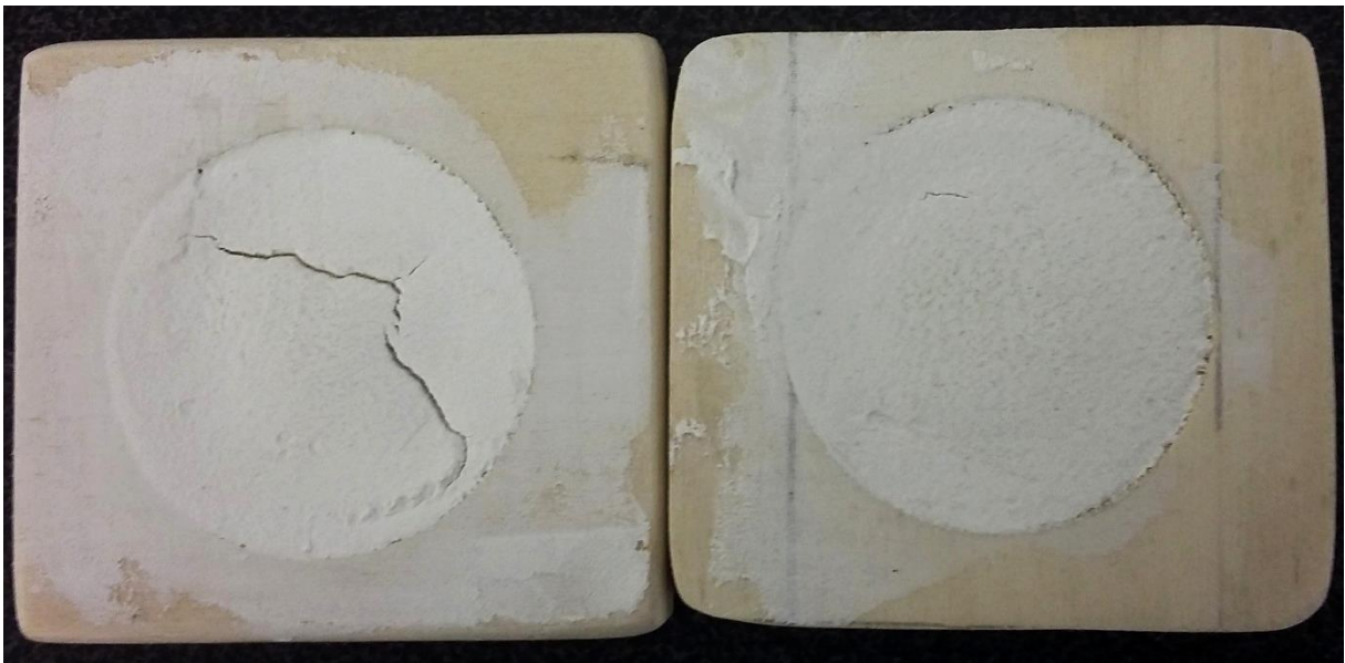
Comparison of the shrinkage behavior of a commercially available dispersion acrylic filler with a layer thickness of 5 mm, once without the addition of Armicell (left) and once with the addition of 0.5% Armicell (right).
