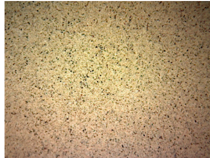
Shrinkage cracking at high layer thickness: 0,75% Armipent 542
