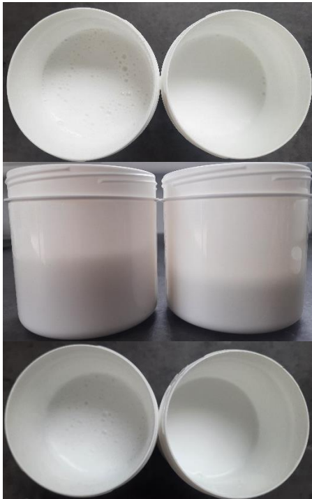
Figure 3: Comparison of foam formation after incorporation into a water-based binder, of Zn-stearate using a dissolver without vacuum (left: Zn-stearate powder; right: Zn-stearate paste).
